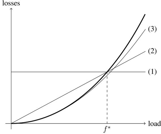
Figure 1. Different models of transmission losses, the thick plot represents the correct physical losses,  $f^*$  denotes the operating point used to estimate the parameters for (1) and (2).
