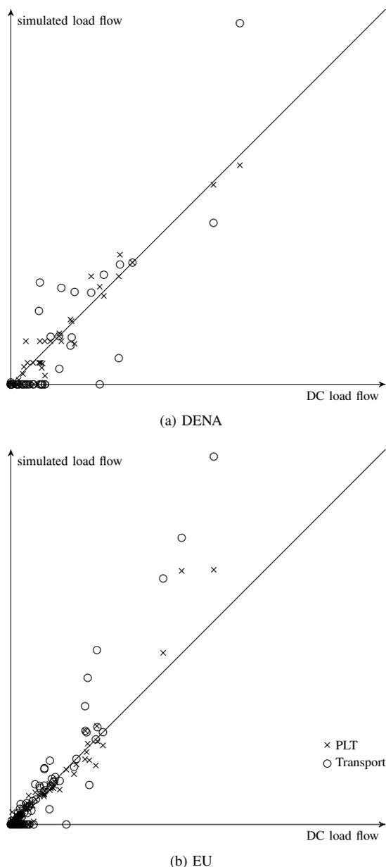
Figure 3. This figure shows load flow values per line for the ED problem. Values both from the PLT and the Transport model are plotted against the reference values (from DC load flow), a dot on the diagonal represents a perfect fit.
